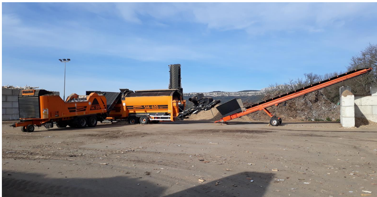
Figure 11 : Installations de broyage – criblage
